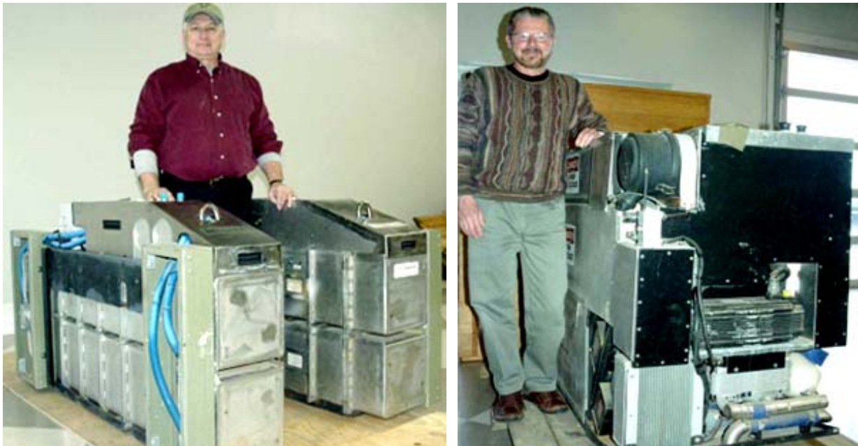
Figure 1. These photographs show the complete and successfully tested metal-hydride storage (left) and 90kW power plant (right) for the underground mine vehicle at our facility in Golden, CO.
