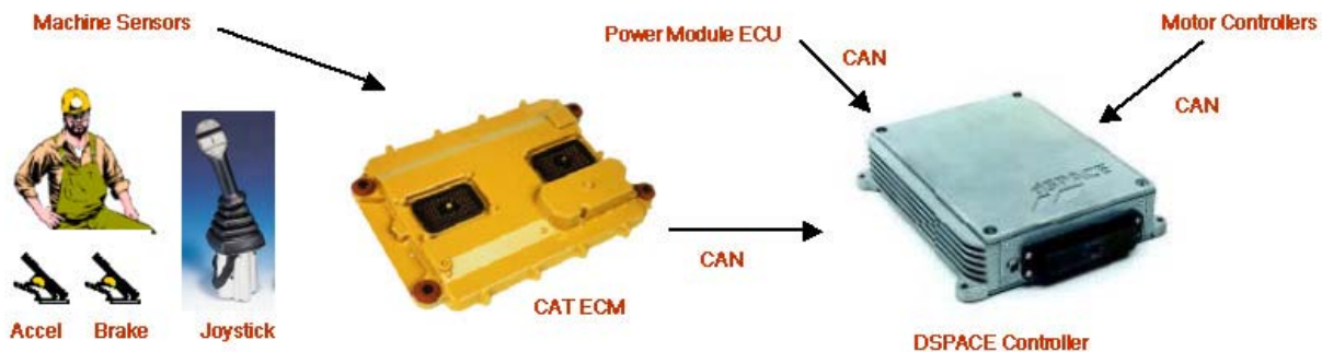
Figure 37: Control logic for the LHD Loader.
