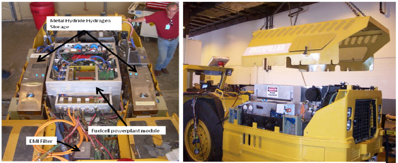
Figures 8 and 9: Fuel cell power plant in situ with storage modules
