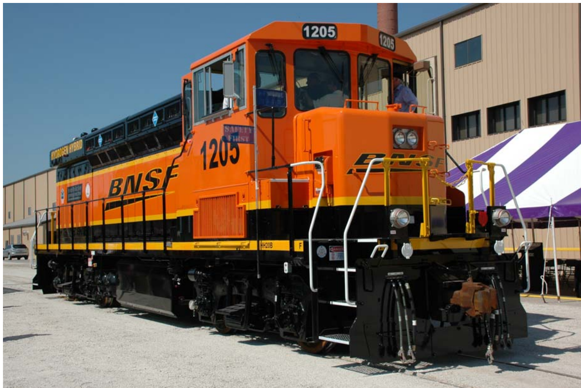
Figure 2: The completed hydrogen-hybrid fuel cell-powered switch locomotive in Topeka, KS.
