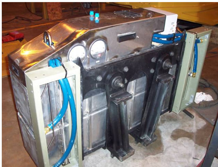
Figure 11: Metal hydrides have high volumetric storage density, long dormancy, reversible operation for very pure hydrogen, and low storage pressure.
