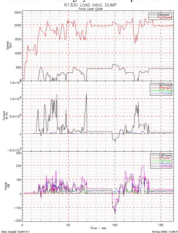
Figure 5: R1300 truck load duty cycle.
