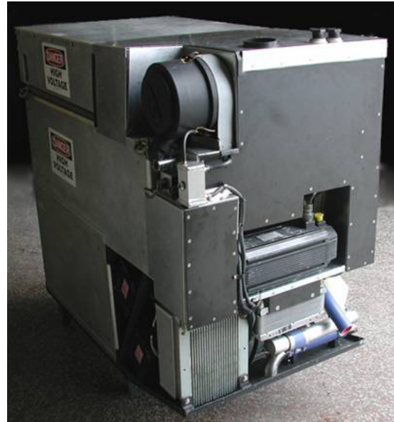
Figures 6 and 7: Fuel cell power plant module uncovered and covered.
