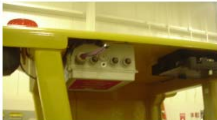
Installed RKI H2 Detection System
