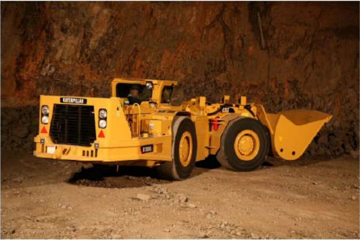
Figure 3. Production R1300 LHD vehicle before the conversion to fuelcell power
